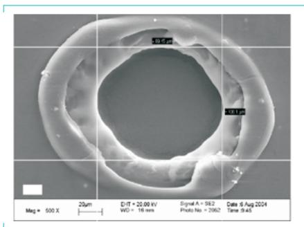
as it requires expensive specialist equipment. It is possible to make holes down to approx. 10  $\mu\text{m}$  thicknesses and up to 200  $\mu\text{m}$ . Laser perforation will typically make slightly oval holes. The advantage of laser perforation is that it is proportionately easy to control the size of the hole.
