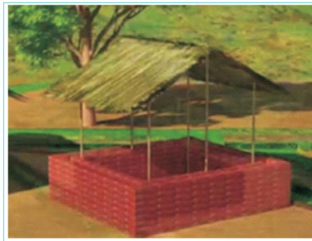
Zero Energy Cool Chamber has been designed by IARI, Pusa, New Delhi on the principle of evaporative cooling i.e. cooling effect created due to evaporation of water.
