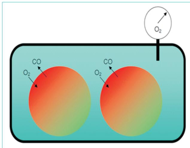
The picture below shows a set-up with respiration vessel and an instrument which measures the oxygen and carbon dioxide contents of the container in which post harvest produce is kept for measuring the respiration rate.
